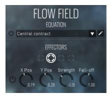
The flow field is defined by a set of effectors and/or an equation as discussed in the *Key Concepts* section of this manual. The circular toggle enabled the flow field equation. The selected equation can be changed with the drop-down menu. To edit the equation, click the pencil icon. For more information on custom flow field equations see Appendix I.
