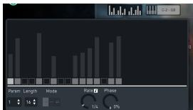
The sequencer editor is a typical step sequencer with every step consisting of a slider with a square toggle below it. The toggle sets whether a particle should be emitted that step, and the slider above it sets a *param*
